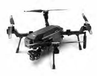
SIRAS is an affordable, easy-to-fly, IP54-rated professional drone with an interchangeable payload system for industrial and utilities inspection, firefighting, law enforcement, and search and rescue missions. With front collision avoidance, hot-swappable batteries, a 31-minute flight time, and no restrictive geofencing, professional UAV pilots can fly safely when and where the mission demands.
